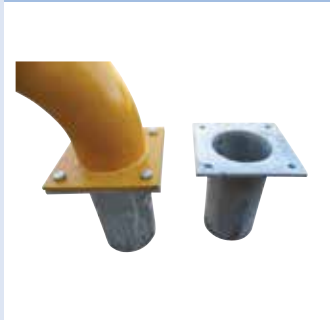
Wheel guide Ø165 mm, 5 mm, 300 mm depth. Mounting plate: 250 x 250 x 10 mm. Weight: 8,5 kg
