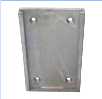
Back plate. Galvanized 450 x 250 x 60 mm Weight: 11 kg Remember rubber spacer
