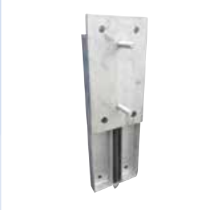
Back plate for 450 mm buffer 750 x 250 x 66 mm Weight: 32 kg Spring loaded. Follows the truck when loading.
